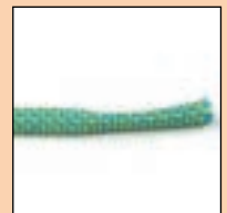
Sheath displacement –core is shorter–
