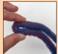
Kink test for assessing rope wear
