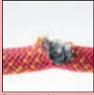
Friction burning —core visible—
