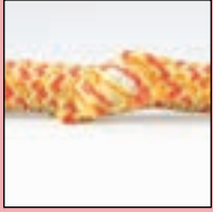
Severe sheath damage
