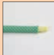
Sheath displacement –sheath is shorter–
